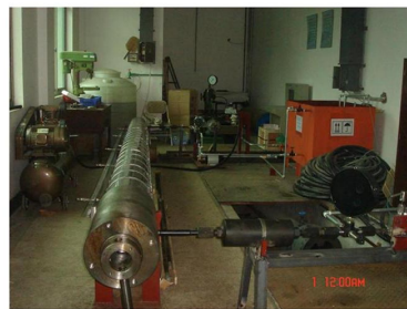
Super-high pressure testing autoclave for CSIC 715 Ø130×5000mm; 200MPa; 250℃
