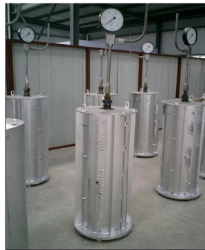
DIA125mm Super-high pressure testing autoclave China Academy of Engineering Physics Ø150×800mm; 180MPa; 425℃ Petroleum University 180MPa; 425℃
