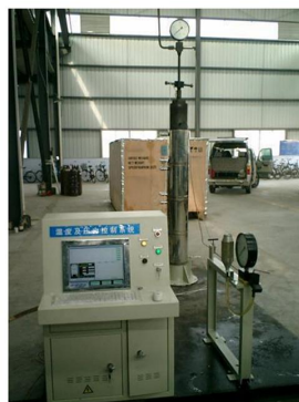
Ø126×1500 Testing device for Xi'an Petroleum University 180MPa; 425℃
